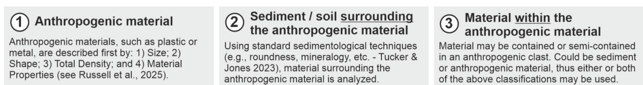
Figure 1. A summary of the three-part methodology for assessing mixtures of sediment and anthropogenic material.
